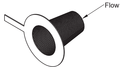
Wire cloth on outside perforated support
